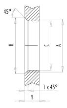
Installation direction: o-ring sits on chamfer.
